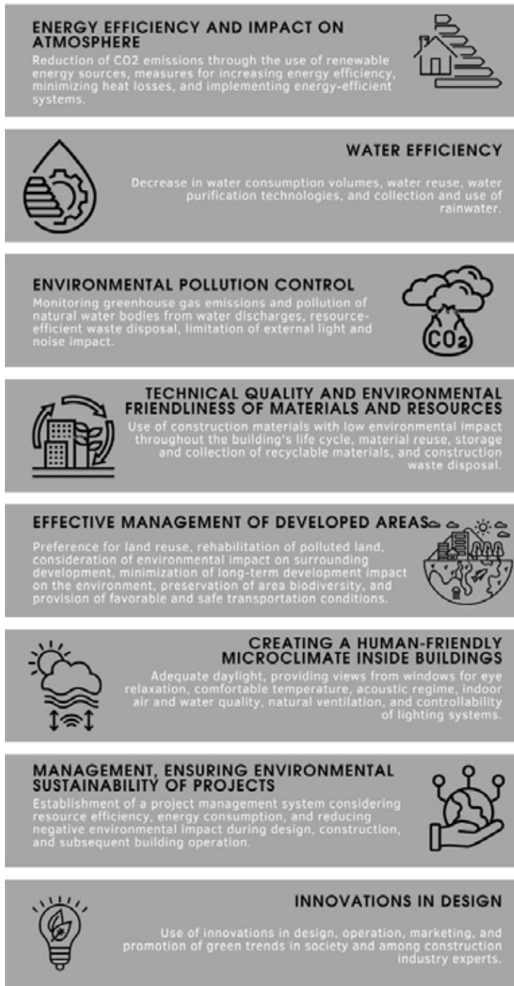
Fig. 1. Categories for assessing the standards of energy and environmental efficiency of buildings (based on voluntary standards BREEAM and LEED)
