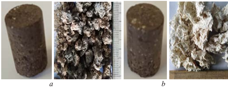
Fig. 2. General view of pellets and their ash residues after combustion made from: a – raw sludge SS-1; b – activated sludge SS-2
